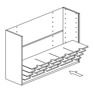
8. To install dividers, insert a divider through each slot. Dividers slide down through slots in all shelves until they rest on the bottom shelf. Note: the end of each divider with the two holes should be facing up.
