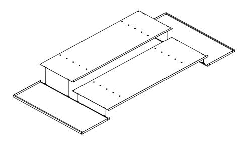
4. Place each of the inside end panels inside the outside end panels, loop side up; the offset lip fits under the flange on the outer edge of the outside end panel. Note: the flange on the inside end panel with the two holes should be facing down.
