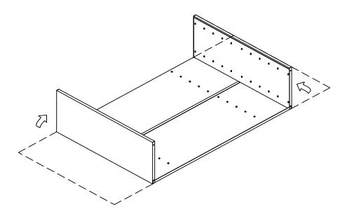
7. To install shelves, begin with the bottom shelf (1" front flange and no divider slots). Position the shelf so its tabs (on side flanges only) lock into the bottom rows of loops on the inside end panels, and its back flange is held by the tabs on the back panel, and set it gently into place. Repeat this same procedure with the four shelves with slots in them.
